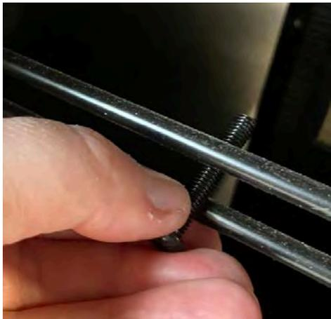
The bolt can be placed through the mounting bracket and then inserted between the the 2 horizontal mesh rails.
