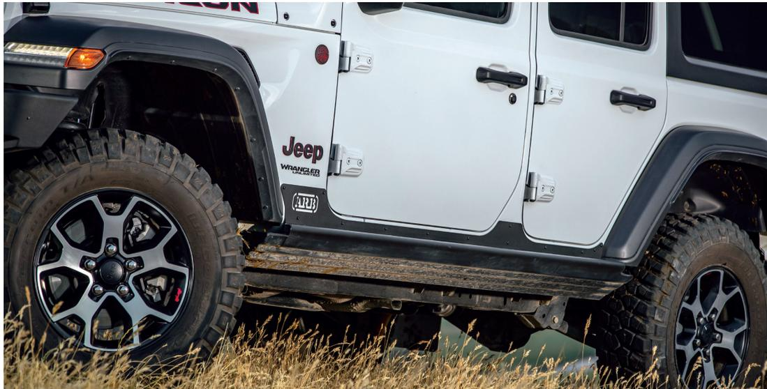
Note: due to slight differences in flare design between the Sport model and the Rubicon, there is reduced clearance between the JL Sport flare and the rock slider.
