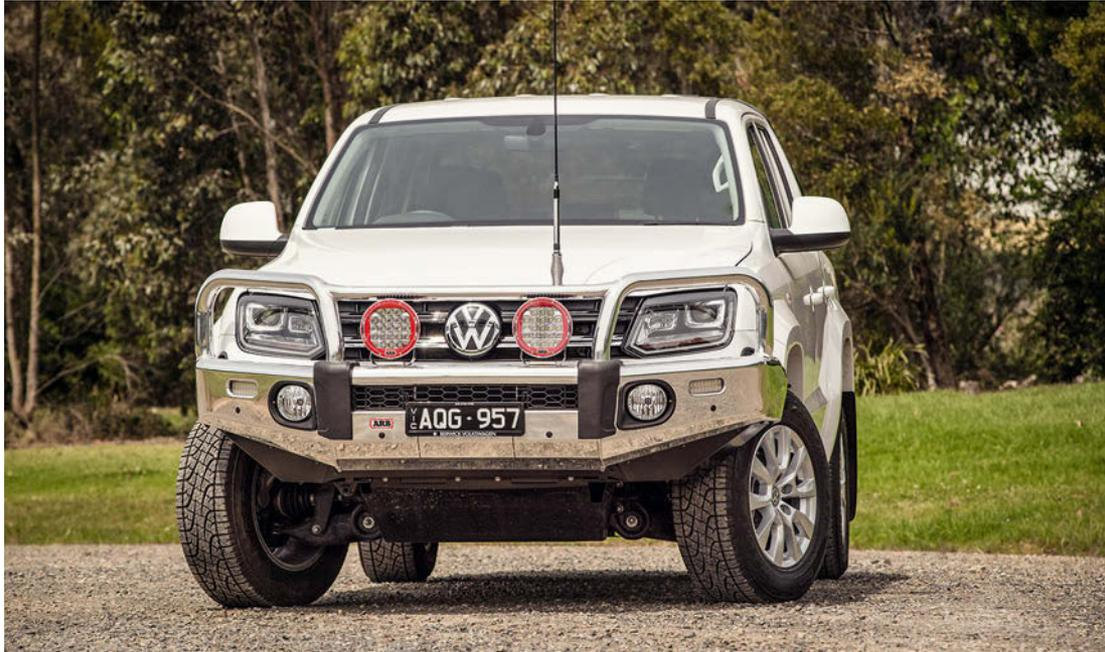
The ARB Alloy bull bar offers yet another choice for frontal protection. With styling elements designed to complement modern four wheel drive vehicles, the bar is manufactured from lightweight and corrosion resistant alloys, with a steel substructure and mounting system for maximum strength.
