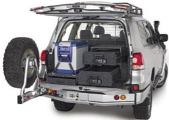
Modular in design for user customisation, Outback Solutions drawers can maximise the versatility of your vehicle's cargo space by being configured with fridge roller drawers, roller floors or stackable drawers. Manufactured from galvanised stainless steel with sealed roller bearings and commercial grade carpet for durability.
